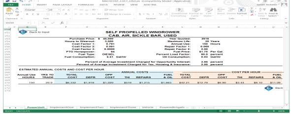
Figure 2. Example Self-Propelled Windrower Cost Summary Table
