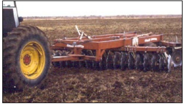
Seedbed preparation usually starts with plowing and disking to destroy previous vegetation, loosen soil, and mix fertilizer into soil. (Photo credit: David Koch)
