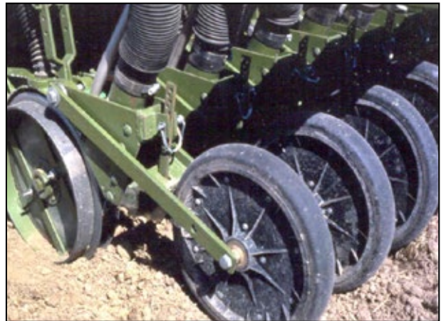
Depth bands (front) and packer wheels (back) help keep drill from placing seed too deep and make good seed-to-soil contact. (Photo Credit: Anowar Islam)
